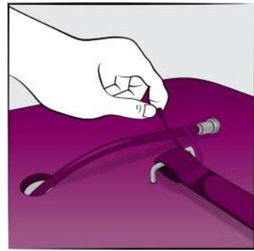
**(Optional):** Use the cable ties to secure the top light cable onto the metal handle on the top.
