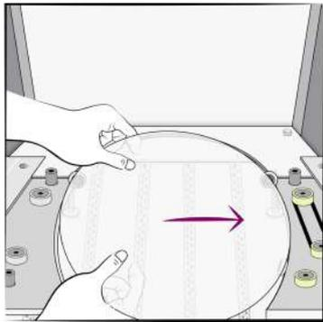
Gently push the edge of the glass platform into the 3 timing pulleys on the spring loaded driving module, then lay the glass platform onto the other end so that it makes contact with the other 2 pulleys and idlers. **Note:** Make sure all pulleys and idlers make uniform contact with the glass turntable platform.
