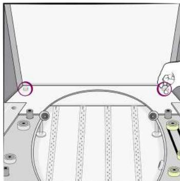
Install the rear bottom division plate, attach 2 small white hand screws. **Note:** Push the rear bottom plate toward the back wall as close as possible, do not over tighten the 2 small white hand screws or else the acrylic will break.
