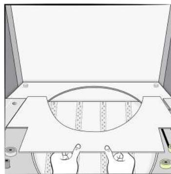
Remove the rest of the acrylic diusion panels from the bottom (back and front).
