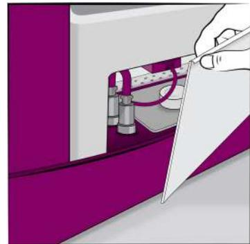
Use the magnetic side cover and cover the openings, one on each side of the turntable base
