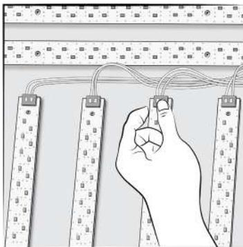
Remove and replace with the new LED lamp. **Note:** The wires and LED lamps are marked V+ and V-. Make sure you plug the V+ wire into the V+ node, and V-wire to the V- node on the LED lamp.
