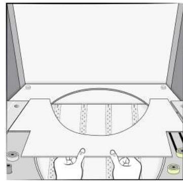
Install the front bottom diusion plate, align the velcro to the ones on the metal frame.
