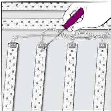
Use a Phillips screwdriver or socket wrench to remove the screw holding the LED lamps node on the LED lamp.
