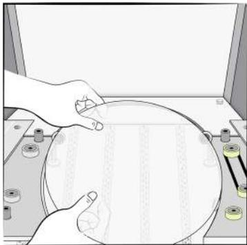
Remove the glass turntable platform if necessary in order to access their respective LED Lamps.
