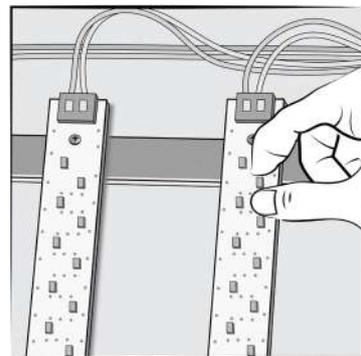
**Caution:** Periodically check for and replace any broken LED crystals in this system. If one LED crystal fails, it can cause others in the same set to malfunction.
