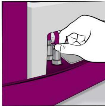
Disconnect the 2 metal connectors for the turntable.
