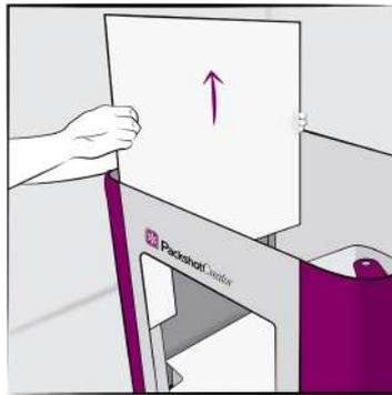
Remove the acrylic side diusion panels, both side walls and front wall.
