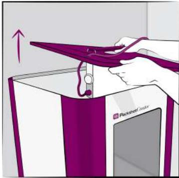
The PackshotStart 360 can be entirely disassembled for easy storage or transportation. Remove the 4 white hand screws and take off the top.
