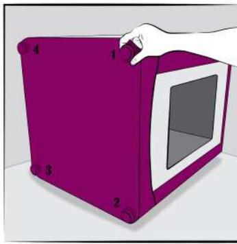
To access the control board, unplug the studio, lay the studio down. Then remove the 4 black hand screws and take off the bottom plate.
