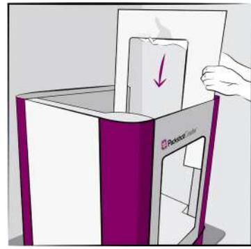
Slide in the panels from the top parallel to the side walls.
