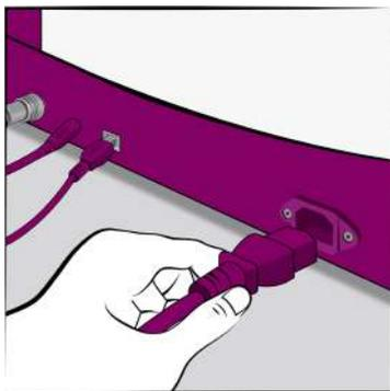
Plug one end of the power and USB cables into the system and the other end into a power jack and computer USB port respectively.
