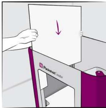
Three acrylic side diffusion panels come with the system – two solid and one with an opening. Choose which two panels to use.
