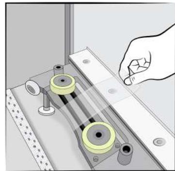
Remove the tape holding the driving module.
