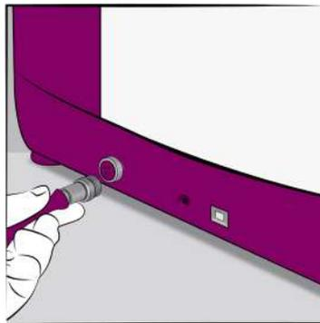
Plug the metal connector into the metal port on the studio.
