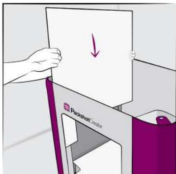
Reverse steps **a** and **b** to install the side walls.
