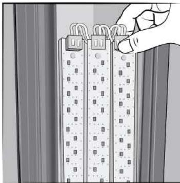
Disconnect the two wires by pressing the connector node while pulling the wire out.
