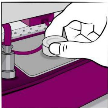
Unscrew the 4 large hand screws holding the built in turntable module.
