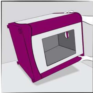
**Note:** Remove the acrylic and glass turntable platforms and tape the driving module down to secure before you proceed to lay the studio down.
