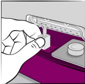
Unplug all the light connections: (turntable, 2 on the front light columns, 4 on the rear light columns.)
