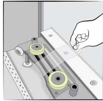
Tape the driving module down to secure.
